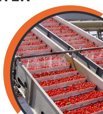
With a double-vision sensor based sorter, equipped with Visible Color and NIR technology (Near Infra Red) the system can detect organic or inorganic foreign bodies, rotten products and color defects.
